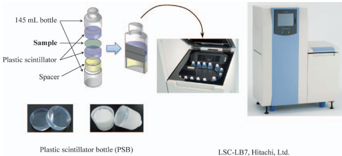
Fig. 3 Assemble of the plastic scintillation bottle (PSB) and low background liquid scintillation counter.
